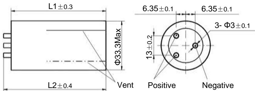
\*Two safety vent on the surface of the case
